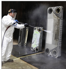
HEAT EXCHANGER CLEANING, SERVICING, & REPLACEMENT
