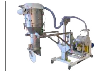
Pneumatic Conveying Systems
